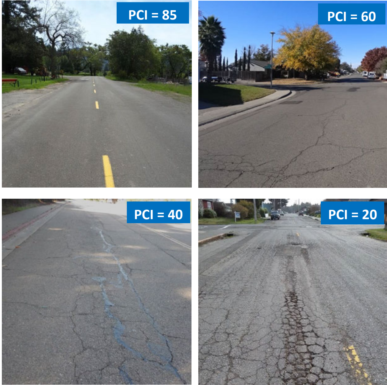
Figure 2. Examples of Streets with Different PCIs
