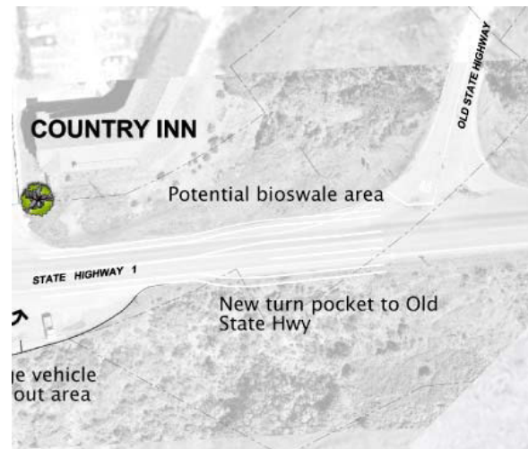
New turn lane at Old State Highway.
