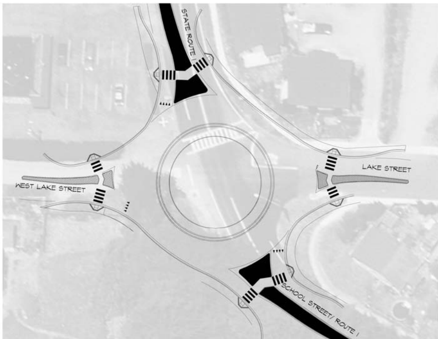
Figure 4-21. Proposed Roundabout at Lake Street/Highway 1
