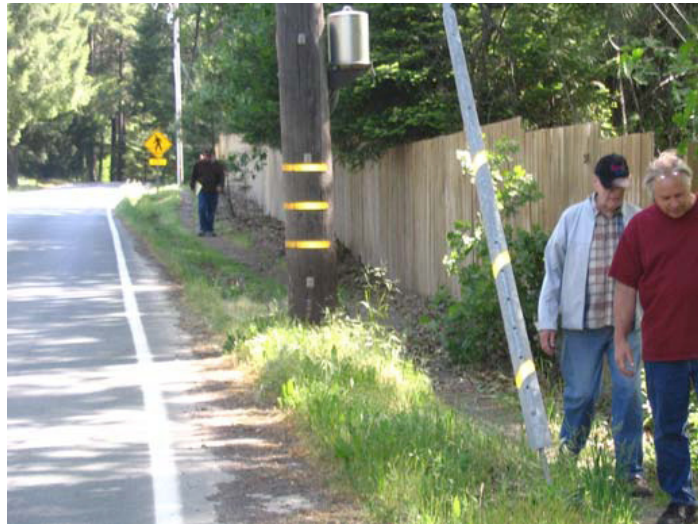
Segment #1 – This photo is taken on the southeast side of Branscomb looking northeast. Although the informal path is well-worn, improving it to a formal walkway may require creative solutions, such as splitting the walkway into two 36-inch walkways around this utility pole.
