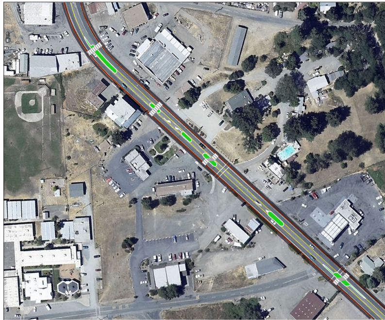
The key locations for crosswalks and pedestrian refuge islands within the Town Center.
